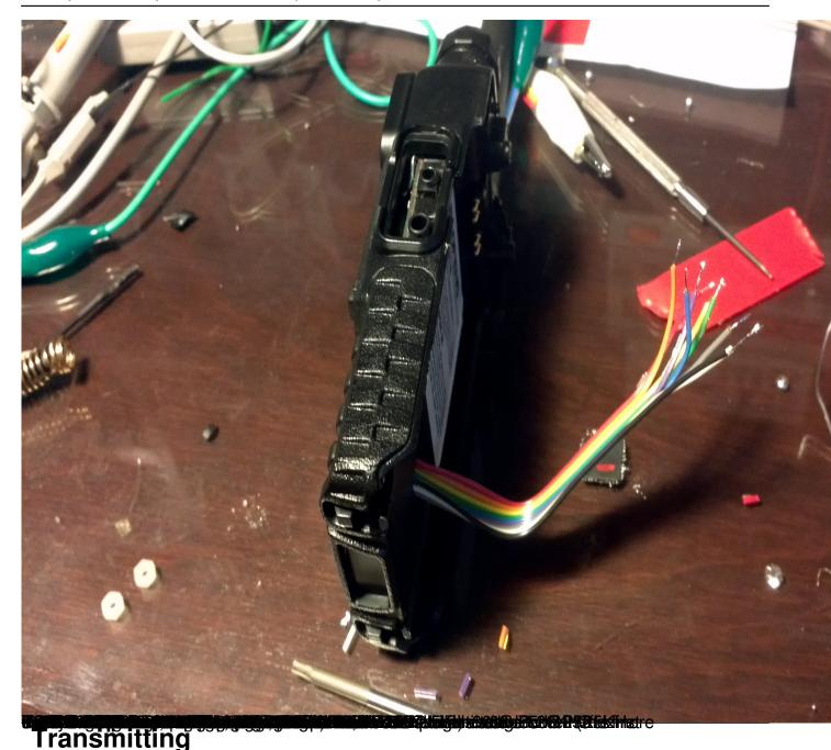
I finally got my license a few weeks ago (KK6BWA) and after messing around a bit with just talking to people, I finally got back to the radio and tried to transmit. I also, tried to read some of the read only registers on the radio, which indicate RX level strength, DTMF decoded tones, etc.
